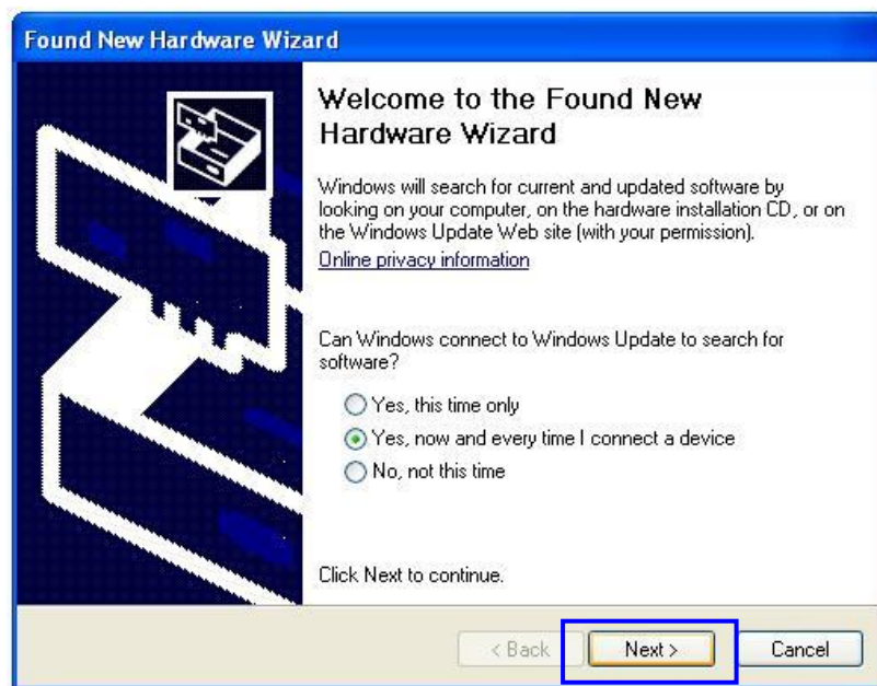
Figure 2-21 Windows XP USB Driver Installation - Step 11
