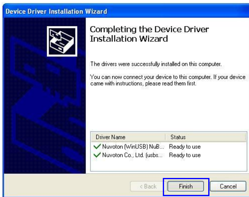
Figure 2-19 Windows XP USB Driver Installation - Step 9
