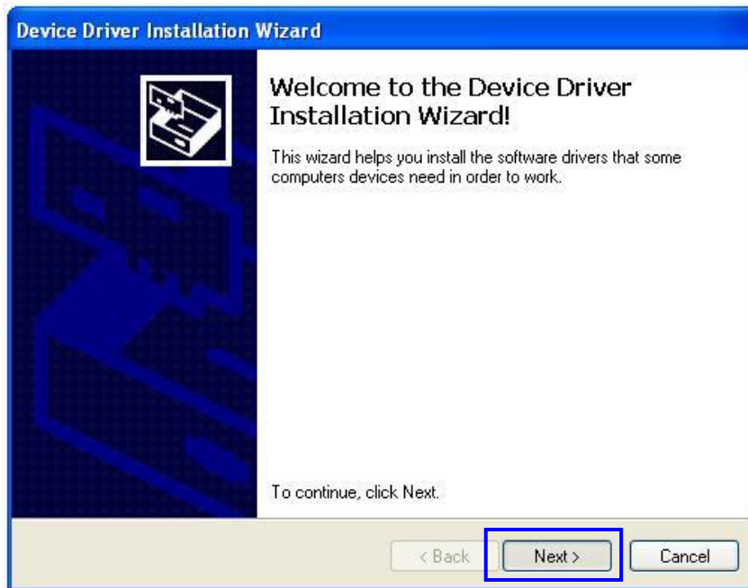
Figure 2-16 Windows XP USB Driver Installation - Step 6
