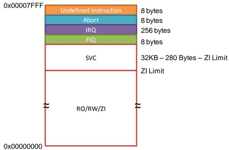
Because the exception handlers of undefined instruction, Abort and FIQ are just forever loops, their stack sizes are all 8 bytes. The IRQ stack size is 256 bytes and SVC stack size is dependent on ZI limit of the program. The stack size definitions are in the startup code and they are as follows:
