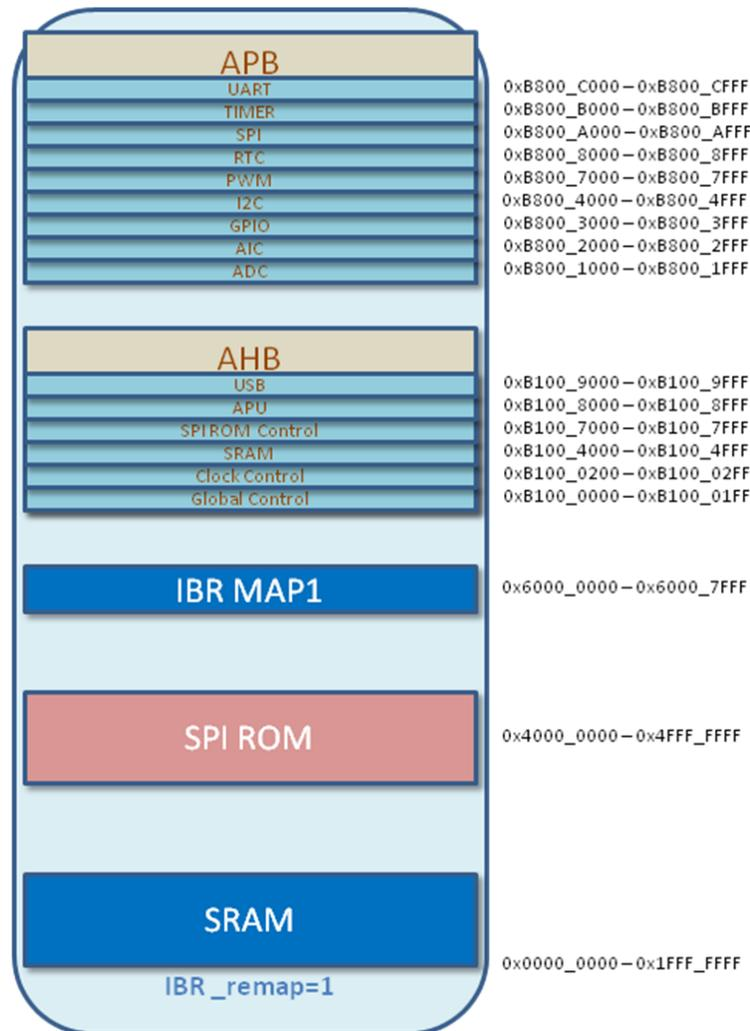
IBR will map the 32KB SRAM to address 0x0 and detect the boot jump setting to boot from SPI, SRAM or USB. If the jump setting is set to boot from SPI, IBR will copy 16KB data from SPI ROM/Flash into the front of the SRAM then set the program counter to 0x0 to execute the code in SRAM.
